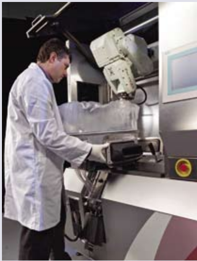
Photo 3: Fully automated molecular processing for clinical use inside a functionally closed disposable unit
