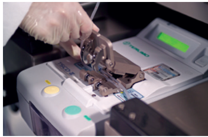
Photo 2: Sterile connections for a closed consumable
