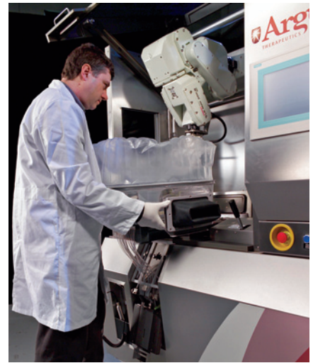
Photo 4: Loading Argos Therapeutics' automated RNA machine with a closed consumable kit
