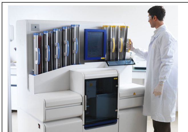
The PREVI Isola automates microbiological processing tasks which have been performed manually for the last 100 years.
